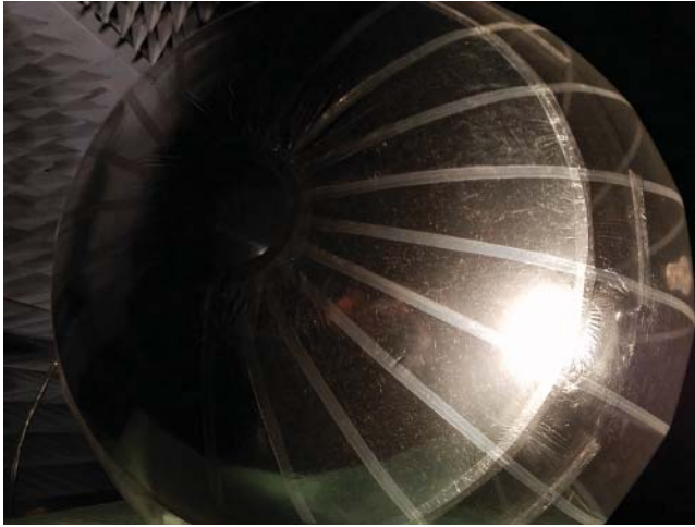
Figure 6.17 Inflatable antenna prototype inflated at Morehead State University prior to anechoic chamber tests.
