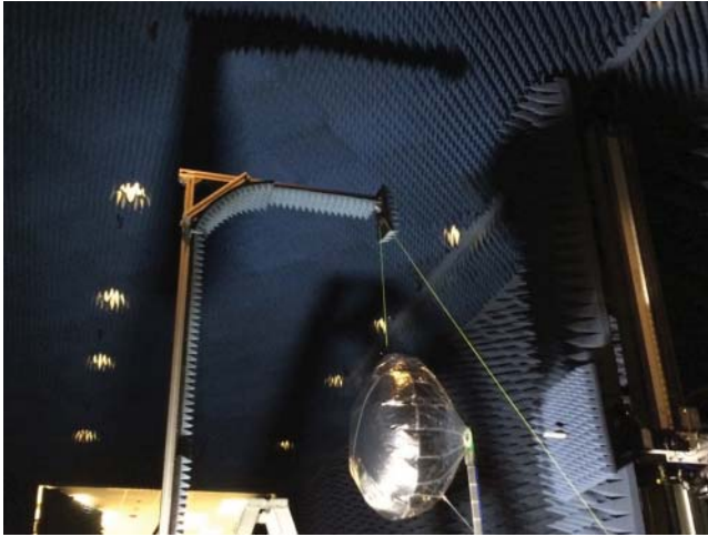
Figure 6.12 Inflatable antenna at X-Band tested at the anechoic chamber of the Jet Propulsion Laboratory. The structure with off-loading mechanism allows the antenna to be pointed correctly.
