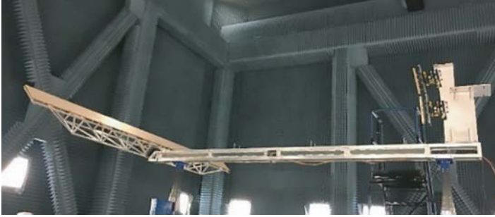
Figure 4.5 Radiation pattern measurement of SWOT's engineering model reflectarray antenna. Courtesy of NASA's JPL/California Institute of Technology.
