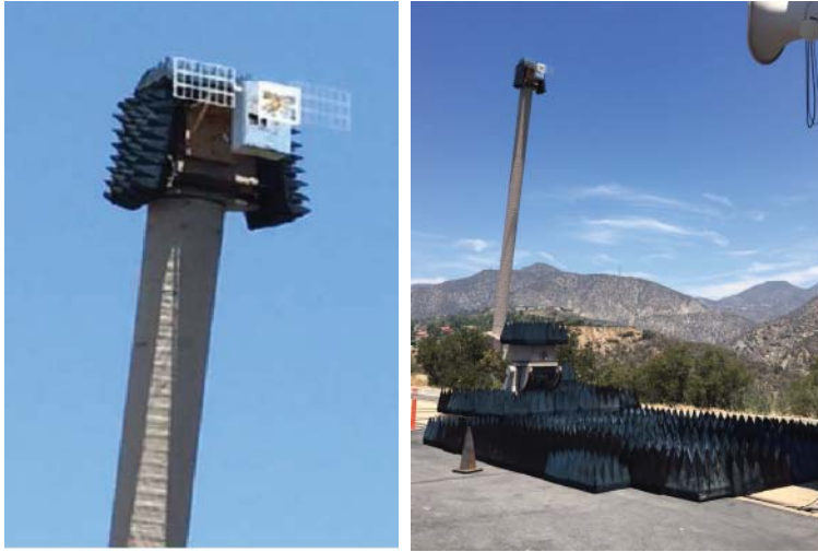
Figure 2.47 West range antenna pattern measurement setup. The antenna under test is placed on top of the post and the ground is covered with absorber material to minimize multi-path interference.
