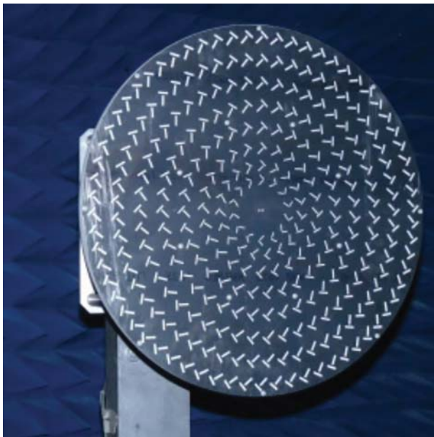
Figure 7.7 Photography of the radial line slot array. Reproduced with permission of IEEE.
