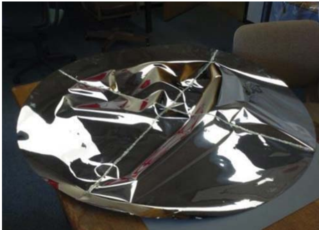
Figure 6.8 Inflatable antenna manufacturing and petals bonding on the reflective side [16]. Reproduced with permission of IEEE.
