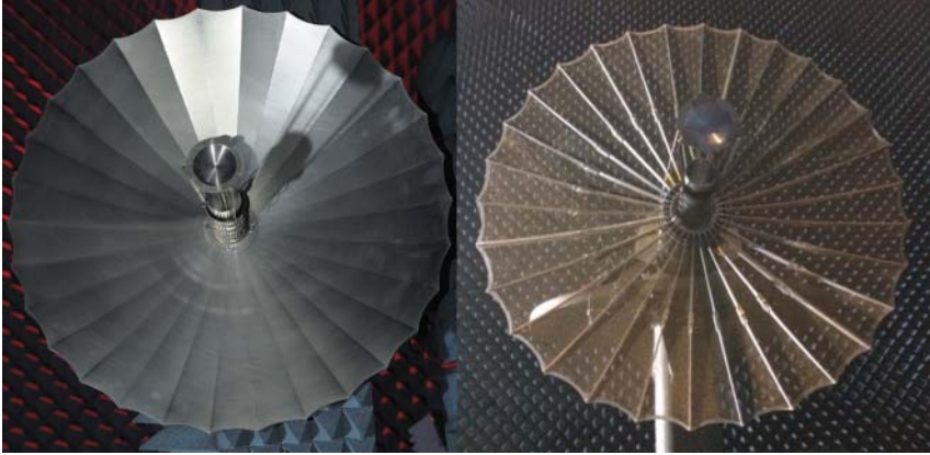
Figure 3.31 Antenna prototypes in the near-field anechoic chamber of NASA’s Jet Propulsion Laboratory: (a) solid non-deployable prototype; (b) mesh deployable prototype.
