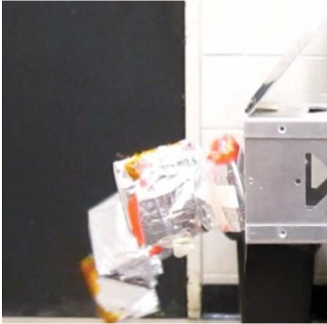
Figure 6.10 Inflatable antenna deployment test [15]. Reproduced with permission from IEEE.
