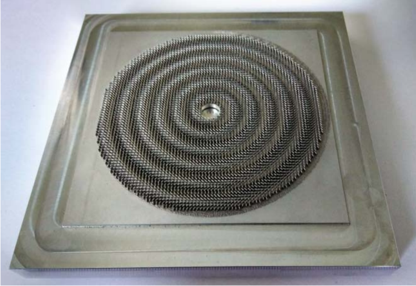
Figure 8.3 Ka-band modulated metasurface antenna fabricated by metal additive manufacturing [32].
