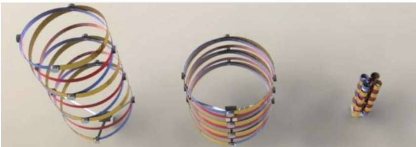
Figure 2.34 Deployable wideband UHF antenna. Courtesy of California Institute of Technology, Pasadena, CA.
