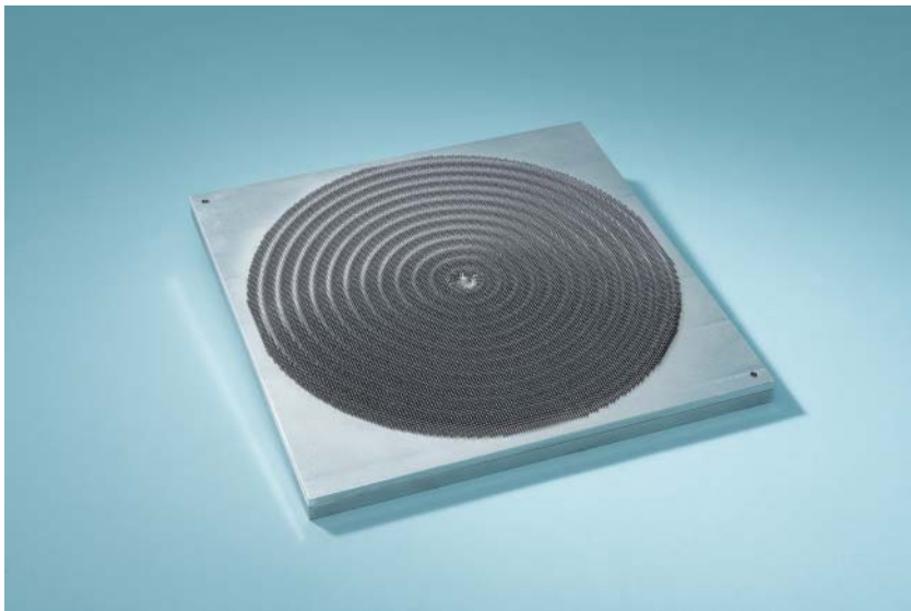
Figure 7.9 Ka-band modulated metasurface antennas fabricated by metal additive manufacturing [16]. Courtesy of NASA/JPL Caltech.
