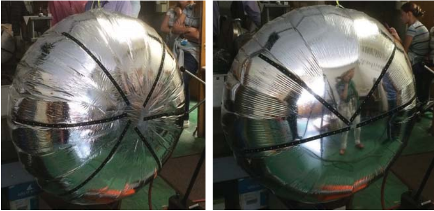
Figure 6.24 A flat surface on the antenna achieved a better surface than a curved surface.
