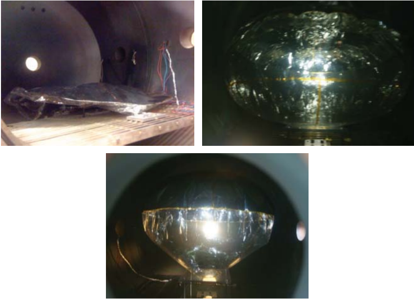
Figure 6.9 Vacuum chamber test performed on the S-Band prototype. The inflatable antenna is vacuumed and inserted in the chamber (a). The cylindrical shape is obtained (b). The conical shape is also obtained (c) [16]. Reproduced with permission from IEEE.
