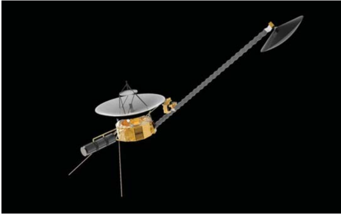
Figure 6.2 Rendering of the concept of a back-up inflatable antenna on board of a larger spacecraft.
