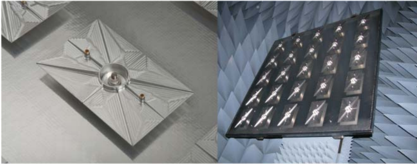
Figure 7.3 The prototype 8 \times 8 patch array designed to survive harsh environment and to achieve high aperture efficiency at both uplink and downlink DSN frequency bands. Courtesy of NASA/JPL Caltech.
