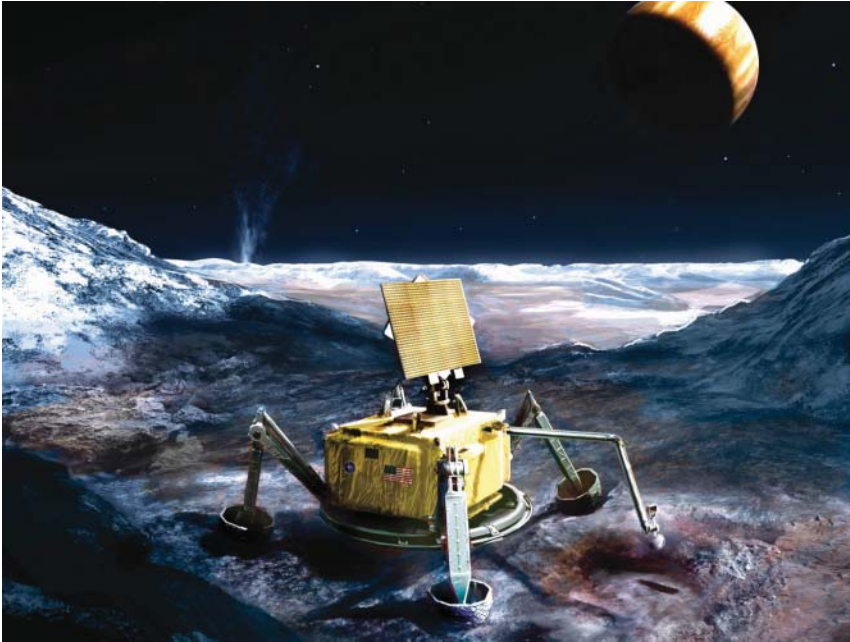
Figure 7.1 An artist's concept of a potential Europa Lander with the all-metal dual-frequency RHCP HGA for Direct to Earth (DTE) communication [3]. This antenna was highlighted as the enabling technology for this mission [3].
