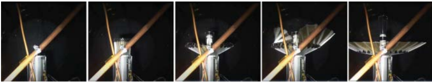
Figure 3.39 Image of deployment in thermal vacuum at 0°C (cold finger and heat exchanger tube in foreground).
