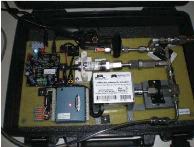
Figure 6.18 Pressure control system developed to maintain the antenna at the desired pressure during the test.
